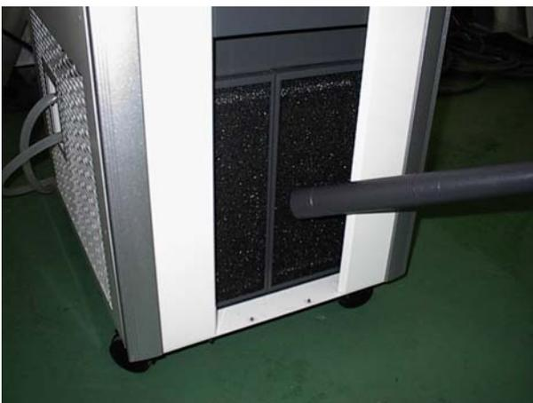
The filter cover is fixed with a magnet. Remove it, and clean the filter or remove dust with a vacuum cleaner. Deep inside the filter is a condenser fin. Do not touch it with bare hands because you may get injured. After cleaning, reversely follow the procedure to replace the filter cover.
