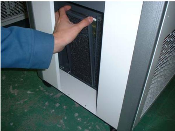
The bottom of the mesh plate is slipped over pins. Lift it up and remove it.
