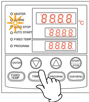
This operation mode is used when “you want to stop fixed value operation automatically after set time since the start”.
