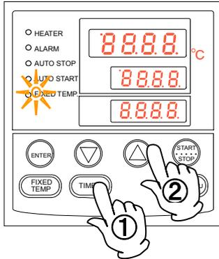
This operation is used when you “want to stop current fixed value operation automatically after several hours”. Quick auto stop operation allows setting the auto stop timer during operation.
