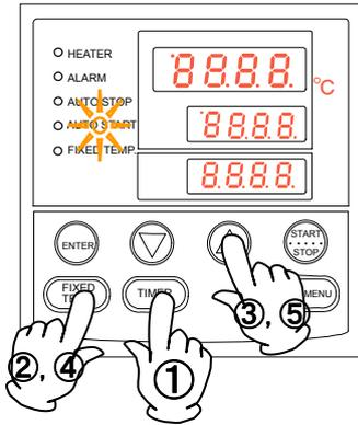
① On the initial screen, press the **Timer** key to blink the characters AStr **AStr** that indicate the auto start operation on the set temperature screen.
