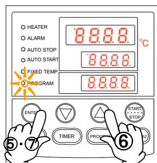
⑦ Press the **Enter** key. The characters Sv-1 **Sv-1** that indicate the set temperature for the step 1 are displayed on the measured temperature display and the current set temperature blinks on the set temperature display.
