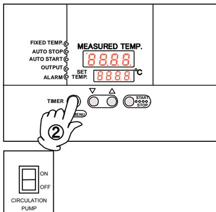
② The activated time of the controller is displayed in the set temp screen.
