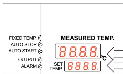
Measured temp screen : Displays the present in-bath temperature
