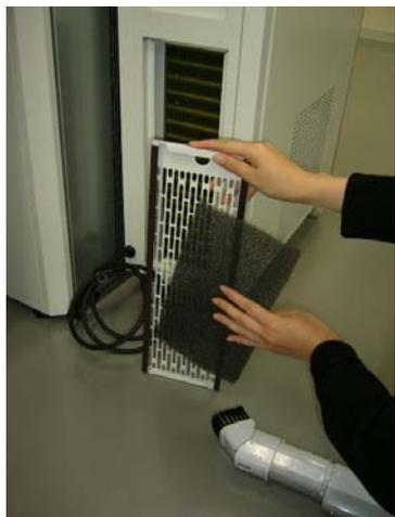
Filter is held with the filter fixing plate. Remove the filter and wash or remove dust with an electric cleaner with the filter attached.
