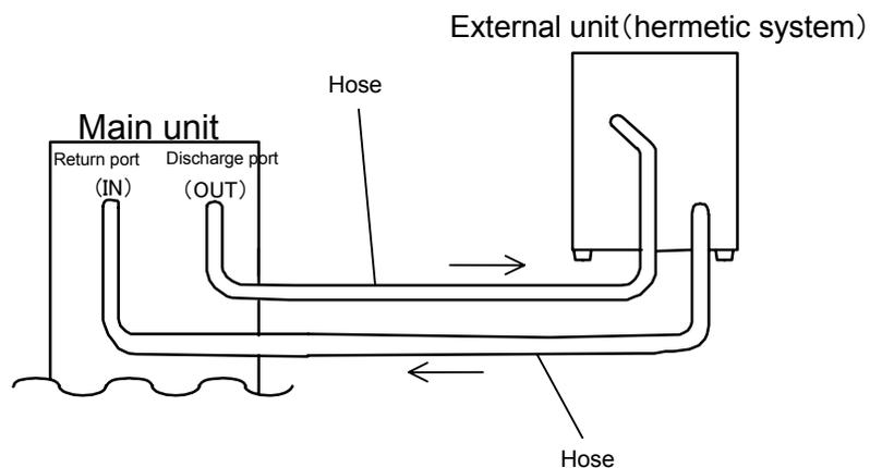
※Attach a hose band and tighten it at the connecting point between the unit and the hose.
