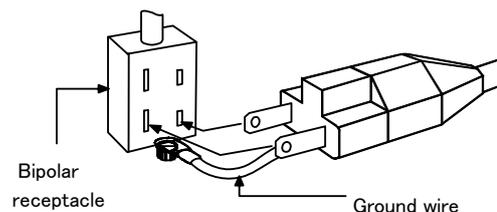
Insert the ground adaptor included as an option, into a power plug confirming the polarity of the outlet. Connect the grounding wire (green) of the ground adaptor to the ground terminal on the power supply equipment.
